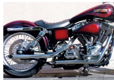
DRAG PIPE MUFFLER for '91up EVO & T/C Dyna (H4240) 1-3/4inch steel / chrome plated comes with "loudly inner silencers" *'91-'94 models require '95 model's genuine muffler bracket
