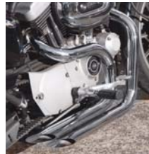
STRING SLASH MUFFLER for '04up XL (H4247) 2inch steel / chrome plated comes with "loudly inner silencers" *not fit forward control models
