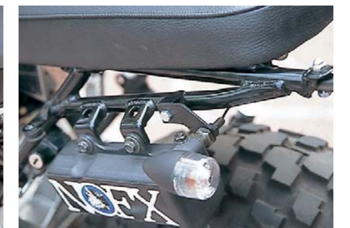
REAR TURN SIGNAL BRACKET (NT0184) steel / black painted fits 8mm or 10mm bolts sold in pairs *not fit genuine turn signals
