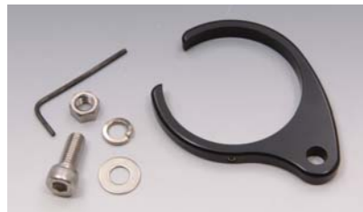
SPEEDOMETER BRACKET for 60mm dia. (5128) billet aluminum / black anodized inner dia.: 61.3mm fits dia.60-61.3mm speedometers fits the speedometer with trip odometer knob
