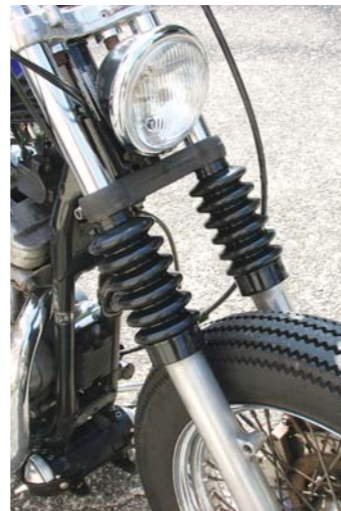
FRONT FORK BOOTS "EASY ON" for 39mm (KIJ0100) sold in pairs comes with cable ties(Lx2, Sx2) *it may not fit long fork chopper or front lowered bikes.
